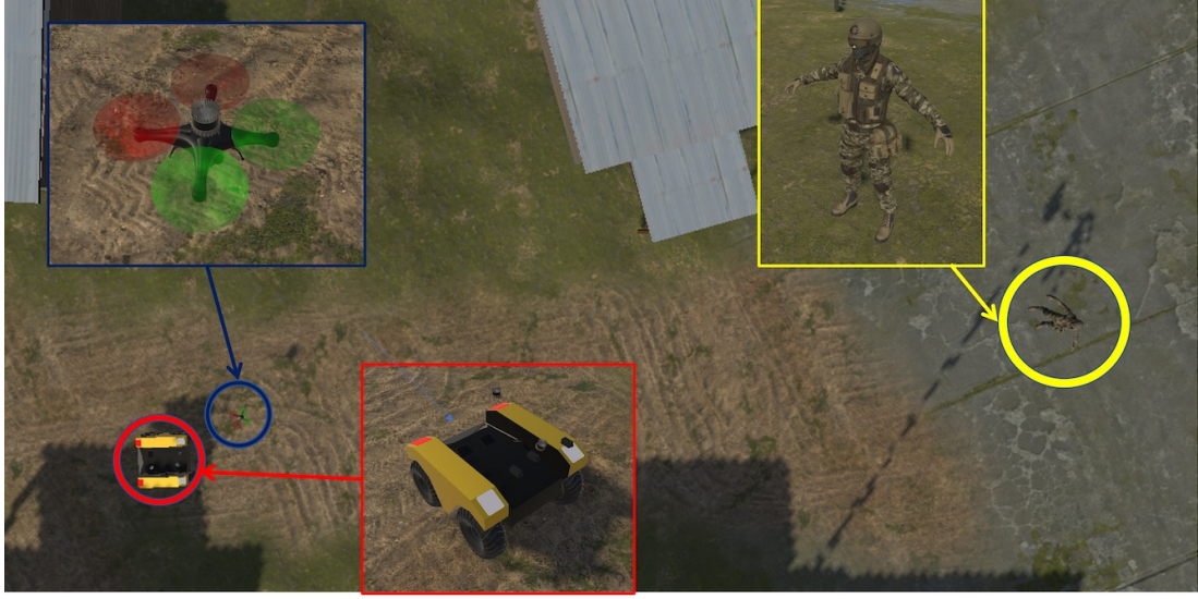
Figure 4.7: Unity-based simulation environment containing an Clearpath Robotics Warthog [2], circled in red, a generic quad-rotor aerial robot, circled in blue, and a target (e.g., soldier model) circled in yellow.
