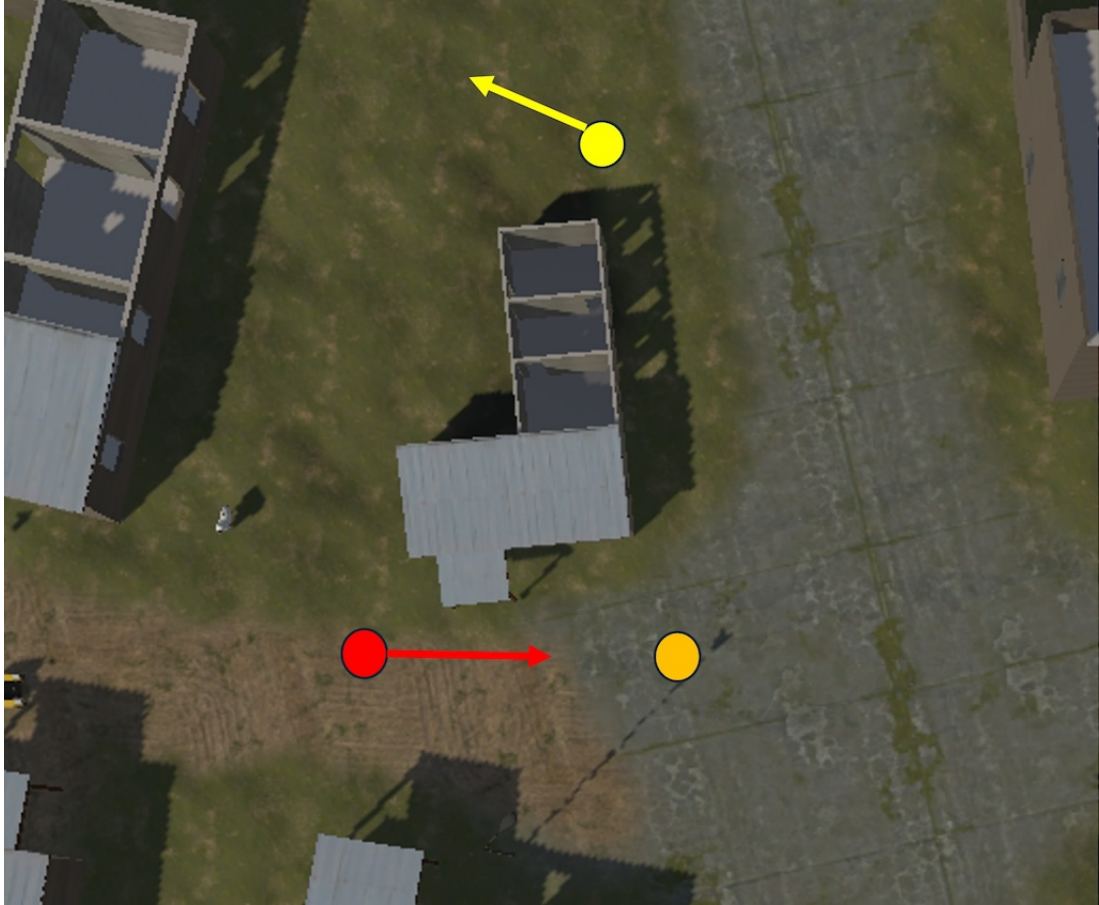
Figure 5.2: The Red circle and arrow indicate the current position and direction of movement of the UGV, which the Yellow circles illustrates this for the target. The Orange circle is the last known location of the target according to the UGV. This large difference in the UGV's knowledge of the target position vs the true position would result in a failure for this run as the possibility of the UGV reacquiring view of the target is minimal.
