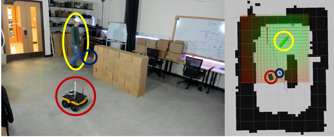
Figure 4.13: Real-world experiment side-by-side with RVIZ containing an autonomous ground vehicle, circled in red, an autonomous micro-aerial vehicle, circled in blue, and a target agent (e.g., a person) circled in yellow.
