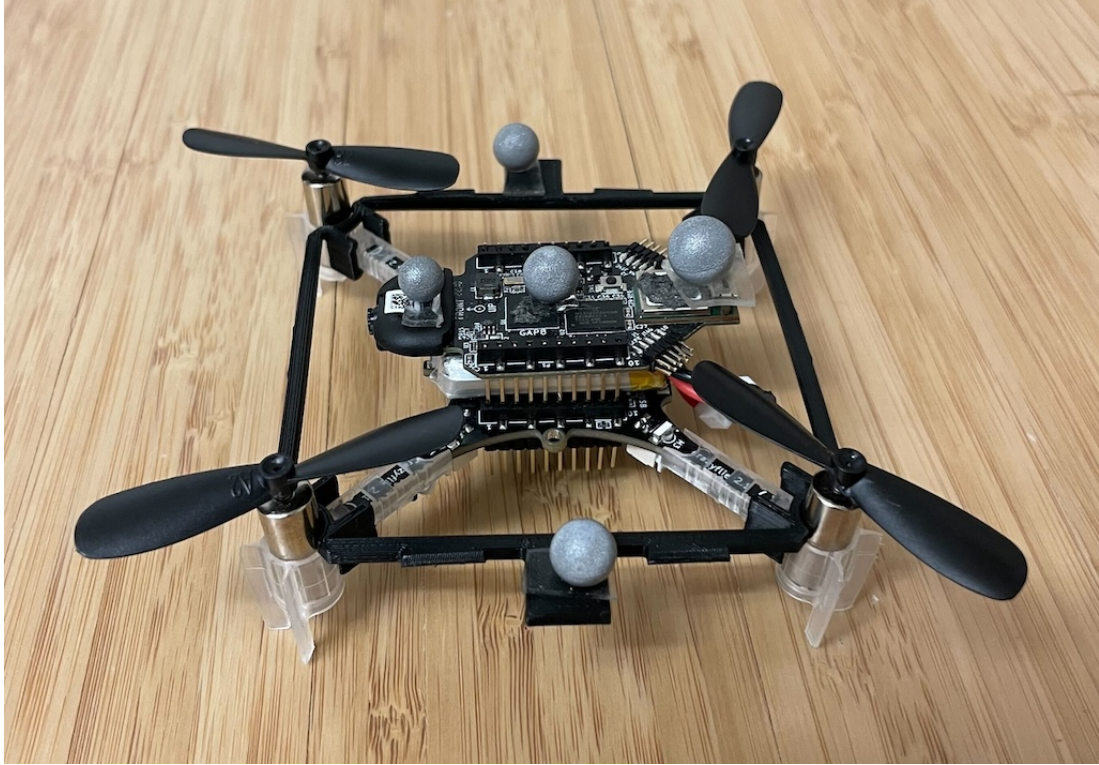
Figure 4.5: Bitcraze Crazyflie 2.1 equipped with their first-party AI Deck with a forward-facing color camera. Also mounted with Optitrack markers for external position and orientation sensing in the lab space.
